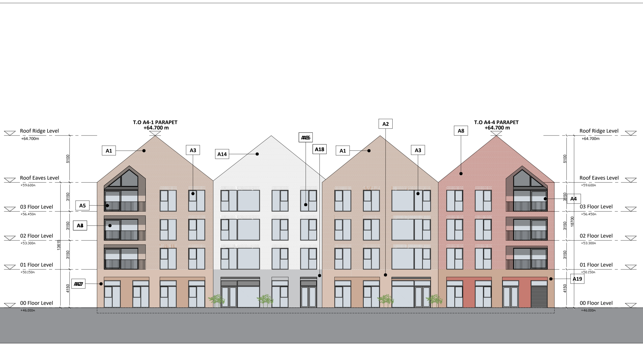
BLOCK 3 EAST ELEVATION 1:200@A1
